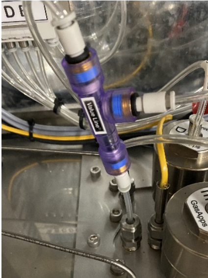
Venturi Valve Attached to Fuse
